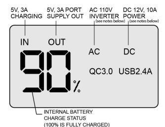
WHICH EVER FEATURE OF THE POWER STATION IS BEING USED THE CORRESPONDING DESCRIPTION WILL APPEAR ON THE LCD SCREEN.
